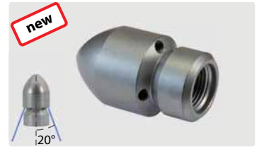
3/8" F. Outside \varnothing 30 mm. 6 rear jets
