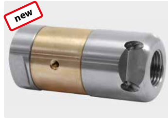
1/2" F. 5 rear jets. 3 side jets. Outside \varnothing 38 mm. ☞ 585 g.
