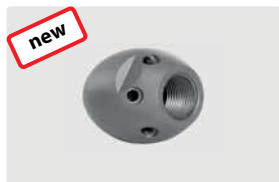
1/4" F. 6x 75° +1x 0°. 20-50 l/min. For \text{R} \text{D} 50-100 mm. Outside \text{D} 30 mm. \text{W} 127 g.
