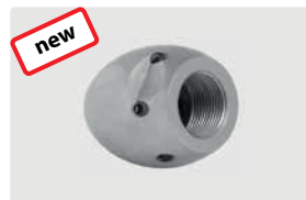
1/2" F. 6x 75° +1x 0°. 30-100 l/min. For \text{R} \text{D} 100-200 mm. Outside \text{D} 40 mm. \text{W} 281 g.
