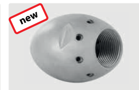
1" F. 8x 75° +1x 0°. 100-250 l/min. For \text{R} \text{D} 150-300 mm. Outside \text{D} 62 mm. \text{W} 1,265 g.
