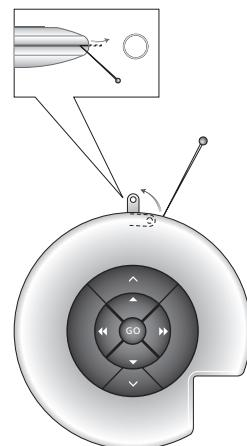
*Use a needle to pull out the key ring tag. You may, for example, use the tag to attach a neck strap.*
