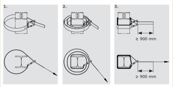
The protective sleeve must cover any edges!
