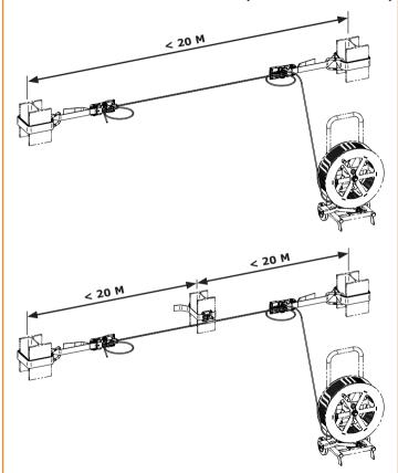
Distances of 20 m or higher require that you install intermediate brackets between the two end points. Field sizes: up to 20 m!
