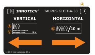
**INFORMATION SIGN:** must be attached at each transition between system sections (VERTICAL  $\leftrightarrow$  HORIZONTAL)
