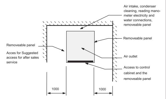
The distance from any constructions blocking the air supply must be at a minimum distance of 1 meter.
