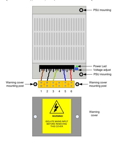
The warning cover must be removed to gain access to the terminal connections. The power supply connections are as follows:
