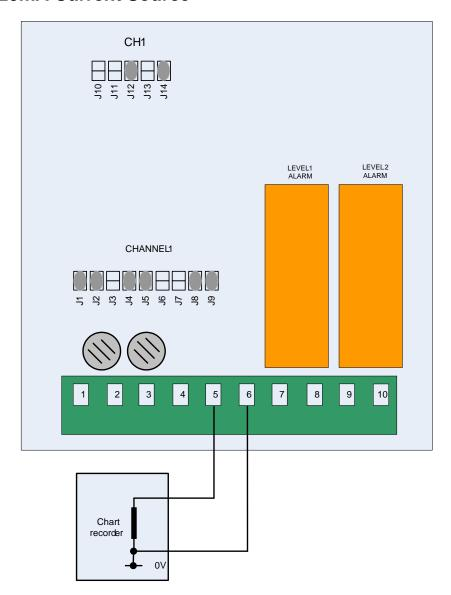
The Input Module sources current proportional to the detected gas level.
