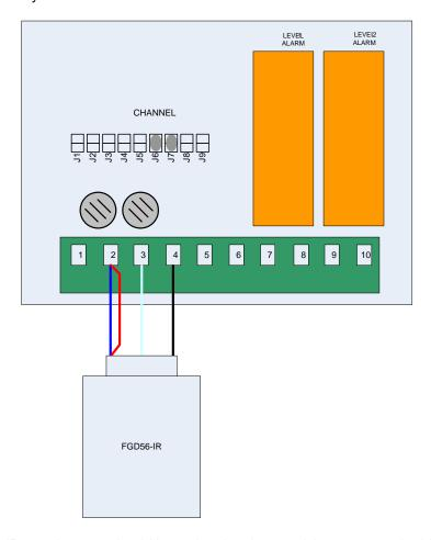
Note: The FGD56-IR gas detector should have the signal set to rising, connect the blue wire to the red wire.
