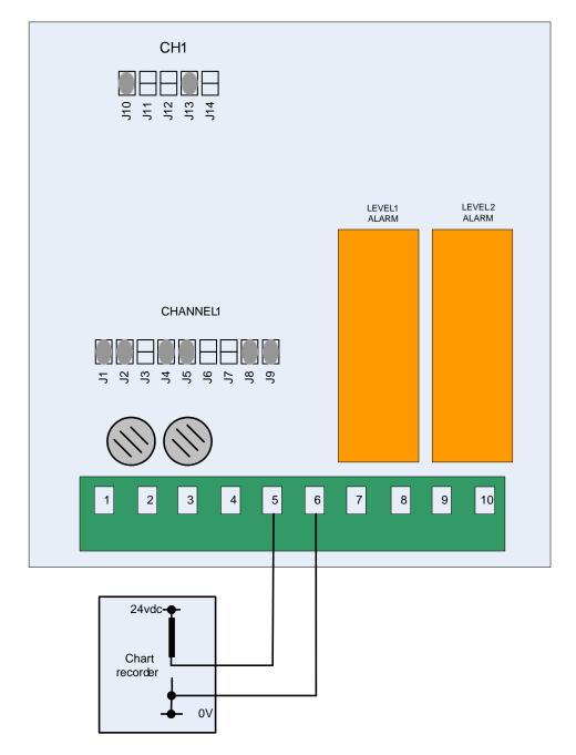
The Input Module can also sink current proportional to the detected gas level.
