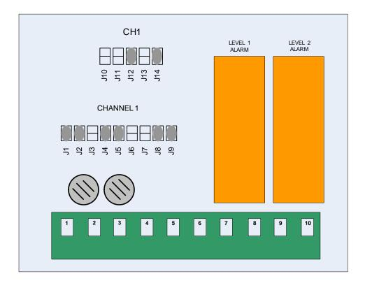
The relay connections shown are with the relay coil in its de-energised state.
