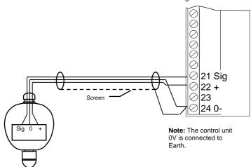
The diagram above shows connection for FGD3 Infrared Detector Head in a non-hazardous location. The pin numbers shown at the control unit refer to pin numbers on the Status Scientific Controls input modules within the MCU Control Units.
