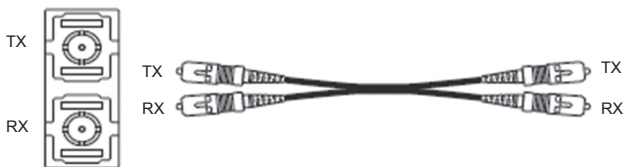
Figure 9 Connection of 100Base-FX Ethernet Port
