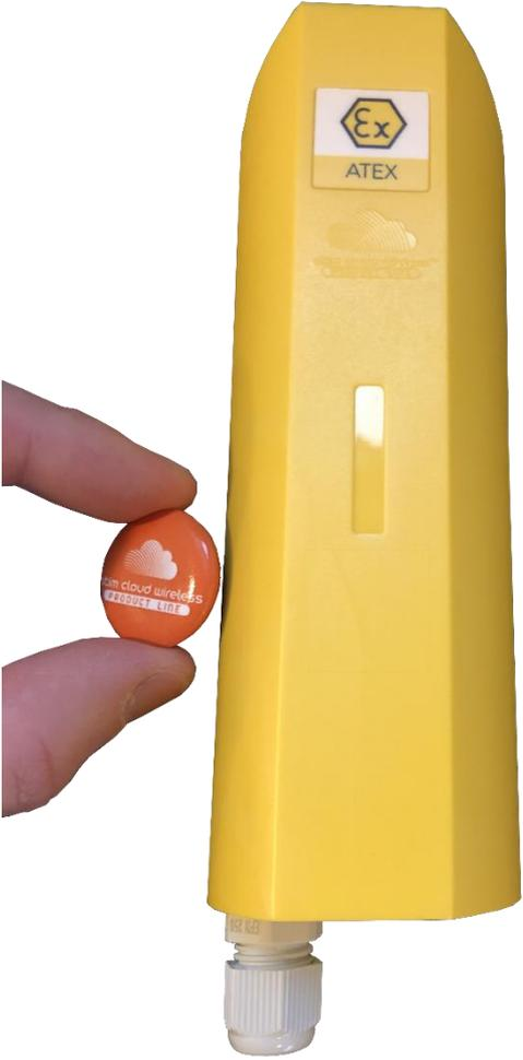
A power failure is achievable by positioning a magnet near a magnetic switch placed on the power supply of the modem.
