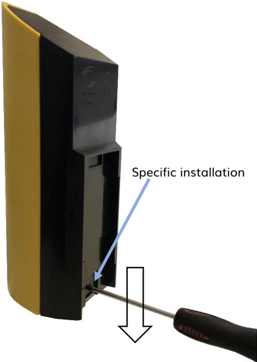
The box must be opened to access the module configuration switches as well as the connection terminal block. To do this, insert the screwdriver in the slot and tilt down to lift the inner tab (see photo opposite). Then pull on the back side to separate the two parts of the case.
