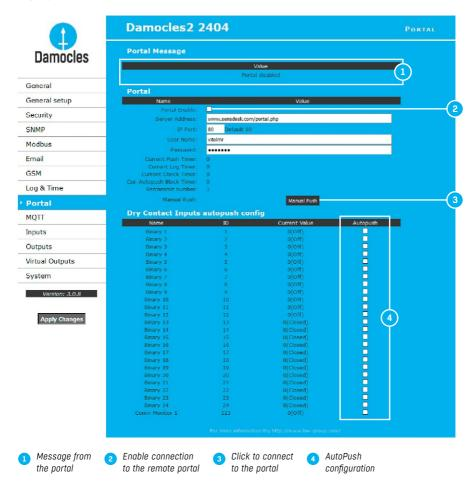
Configures the communication with the portal using the HWg-Push protocol. Damocles2 is the active side and establishes the connection periodically and/or whenever a change in a sensor value exceeds the configured AutoPush value.
