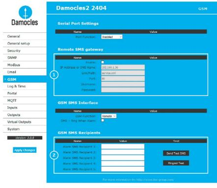
1 IP address of "HWg-SMS-GW" to use for sending text messages (SMS)
