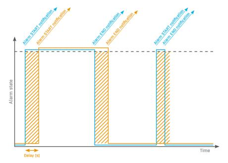
Alarm status notification based on a Delay value:
