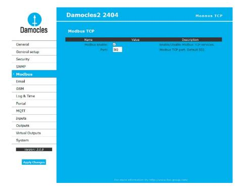
**Note:** The Modbus/TCP protocol is not secured in any way. We do not recommend using it outside of an isolated network. For basic security, it can be combined with the IP address filter.
