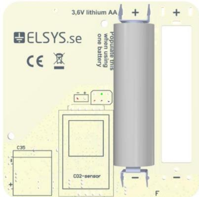
3. Mount the back panel to the wall with at least 2 appropriate screws, using any of the four mounting holes. Alternatively attach the sensor using double sided adhesive tape
