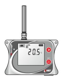
This model is equipped with only one internal temperature sensor, no additional probes and sensors can be connected. It is characterized by a simple and compact design and a relatively long response to a temperature jump. The device is placed directly in the measured space. During the charging period the measurement accuracy may be affected by up to 1 °C due to parasitic heat .
