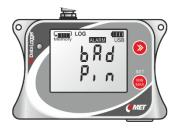
The SIM card requires a PIN code, but the PIN is not set/enabled in the SW configuration (Default).
