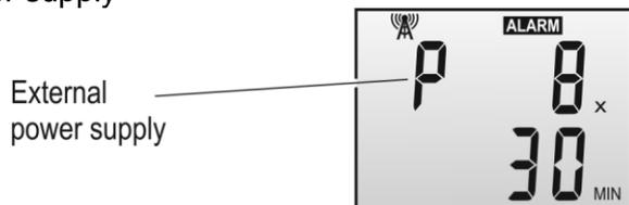
**P (Power)** – information about presence of external power supply is refreshed with interval of 1 min.
