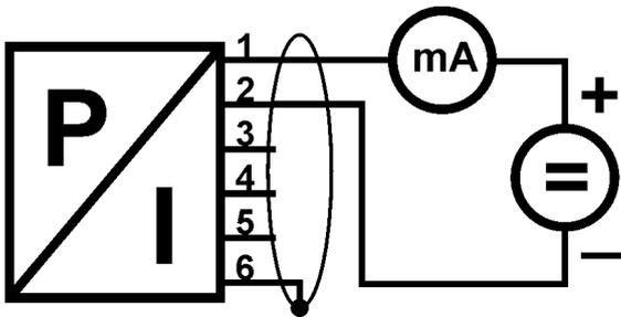
**F** 4 - 20mA two-wire is most common analog output. Minimum supply voltage is 5V. Transmitter has its software and hardware max. current limitation in loop.
