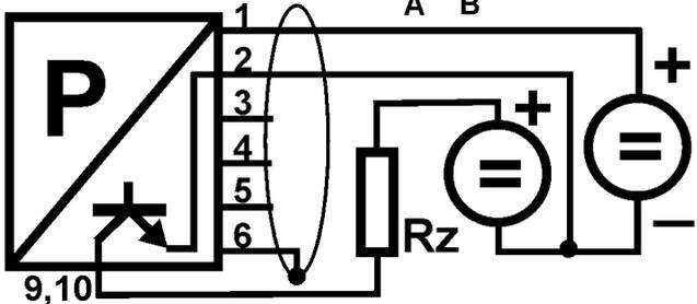
**L** is double switching output with NPN transistors with open collector. It is possible to switch by current up to 100mA and DC voltage up to 50V. Load can be simple resistor, bulb, LED, relay etc.. Load is always galvanically connected with transmitter supply. Transmitter power supply and load power supply can be shared. Switching levels, hysteresis, polarity are setting by software. It can be also set switching „window“.
