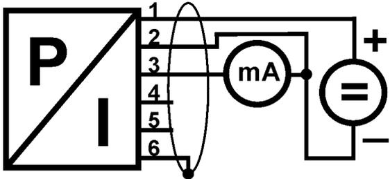
**G** 0 - 20mA three-wire. Can be set on 4-20mA range. Maximum load impedance  $R = (U_{cc} - 2) / 20\text{mA}$
