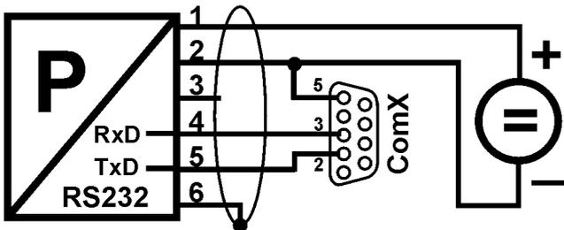
**A** digital output RS232. Can be connect directly to native or mapped (USB, LAN) serial port. For communication are used data signals Rx and Tx. RS232 line is not galvanically isolated.
