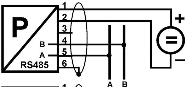
**B** connection on RS485 bus. Device address can be assigned in range 00 to FF and can set other communication parameters. Line is not galvanically isolated, when the power supplies from various sources is recommended to interconnect their grounds.
