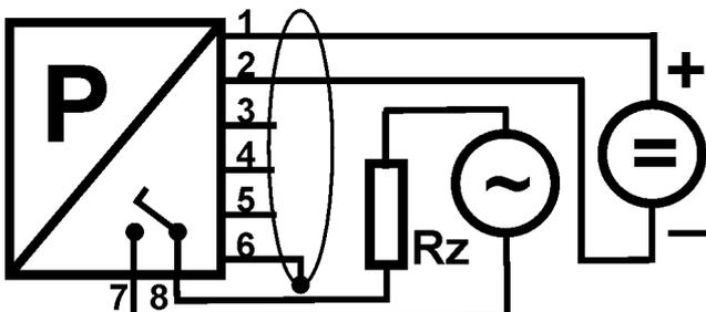
**R** is switching output with galvanically isolated contact bistable relay. It is possible to switch DC and AC up to 40V and max. current 0,5A. Switching levels, hysteresis, polarity are setting by software. It can be also set switching „window“.
