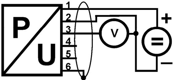
**H** 0-10V, can be also set different ranges. For ranges smaller than 3V is recommended to switch transmitter output range for resolution D/A converter. Min. supply voltage has to be 2V higher than max. output voltage. Max. current load is 20mA
