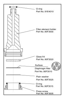
Screw the press screw by hand into the filter element holder up to the diaphragm filter.
