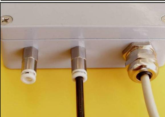
Connection by means of plug couplings. It is precise with guaranteed seal and pressure resistance up to 1MPa. Code parking **N** for tube with the outer diameter 4mm, **M** for tube with the outer diameter 6mm. The material is nickel plated brass and plastic, sealing O ring NBR.
