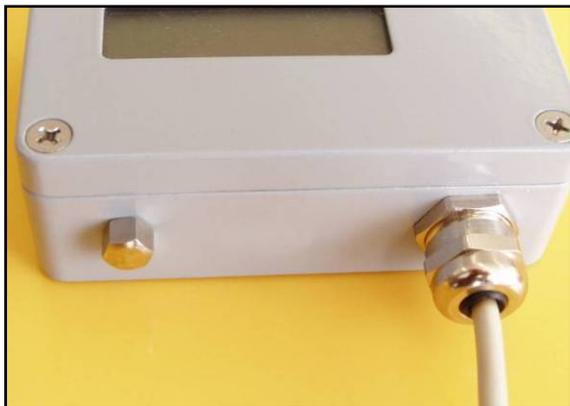
For measuring barometric pressure – marking **B** – the inlet hole is protected by a metal cover from nickel plated brass. Obviously, it is possible to equip a transmitter for measuring barometric pressure with any of the above mentioned fittings.
