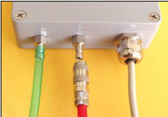
Basic pressure connection with the code **R**. It is used as a nipple for a quick coupler or an outlet for direct sliding on a tube for pressures smaller than 100kPa. The outer diameter is 5mm, the material is nickel plated brass.
