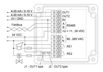
To use analog outputs, connect the terminals OUT1 and/or OUT2 and OV to the input of the secondary instrument (indicator or controller). NB! The outputs are not galvanically isolated from 24 V power supply and share common OV. Allowed load resistance limits are stated in Specifications table.
