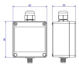
E2228 provides two independent analog outputs OUT1 and OUT2, user-selectable to 4-20 mA or 0-10 V, proportional either to humidity, temperature or dew-point value. RS485 Modbus RTU digital communication interface allows easy instrument configuration and integration into various automation systems.
