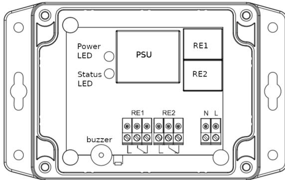
The terminals on the E2630 series devices are suitable for a wide range of wires with cross-section 0,2...1,5 mm<sup>2</sup>. We recommend to strip the wire end by 5...6 mm and use the wire end sleeves. To connect the wire, loosen the screw, insert the wire end into the terminal hole and tighten the screw. The outer diameter of the cable must not exceed 8 mm.
