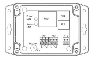
The terminals on the E2630 series devices are suitable for a wide range of wires with cross-section  $0,2...1,5 \text{ mm}^2$ . We recommend to strip the wire end by 5...6 mm and use the wire end sleeves. To connect the wire, loosen the screw, insert the wire end into the terminal hole and tighten the screw. The outer diameter of the cable must not exceed 8 mm.
