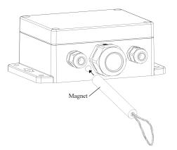
A short touch (< 2 s) enables the automatic mode, a touch of 2...10 s - manual mode. The activation of the automatic mode is followed by a single LED blinking and acoustic signal. If manual mode is activated, the double acoustic and light signal follows.
