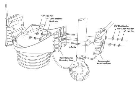
If you wish to put the anemometer higher than the rain collector side of your ISS on the support tube, follow the instructions in the ISS Installation Manual for mounting each side *separately*.
