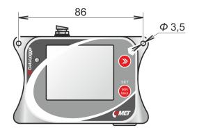
• You can fix the device on the wall with the aid of a lockable holder LP100 (optional accessory)
