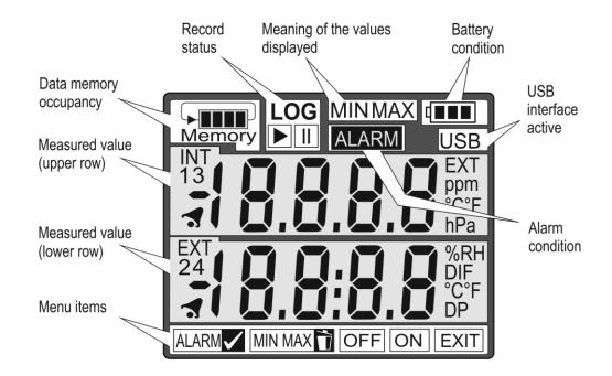
**Data memory occupancy** - this display section offers information about the current condition of the free space existing in the data memory. The blinking of the *Memory* symbol indicates that the preset memory occupancy limit has been exceeded. This limit can be set up in the device's configuration. Several actions can be assigned to it (optical and acoustic signalling).
