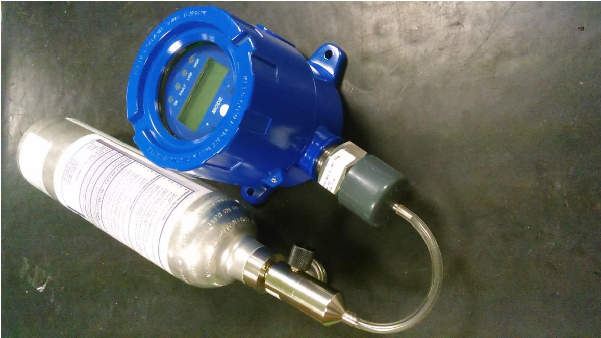
Sensotox 2 connected to a calibration gas cylinder with an adapter.
