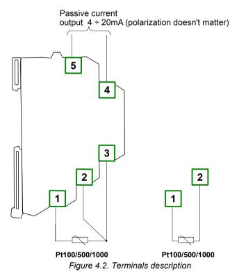
Temperature sensor can be connected to the device in typical 3-wire circuit (Figure 4.3a) or 2-wire circuit (Figure 4.3 b). Due to precision of measurement 3-wire circuit is recommended.
