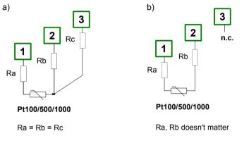
Figure 4.3. Connection of sensors: a) 3-wires circuit; b) 2-wires circuit;
