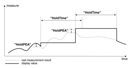
Figure 5.1. Process of peaks detection
