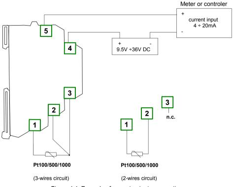
Figure 4.4. Example of current outputs connection
