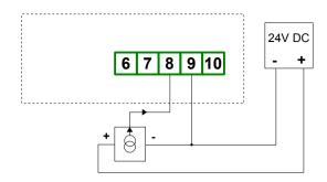
Figure 4.8. Connection of 3-wire current converters
