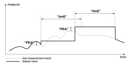
Figure 6.3. Process of peaks detection
