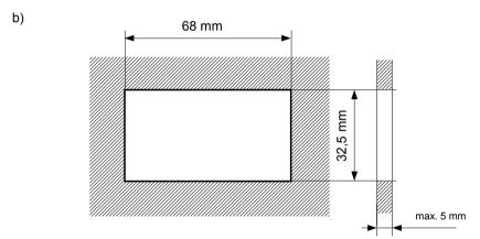
Figure 4.1. Mounting hole dimensions: a) recommended b) allowable
