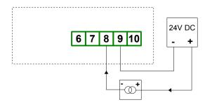
Figure 4.7. Connection of 2-wire current converters
