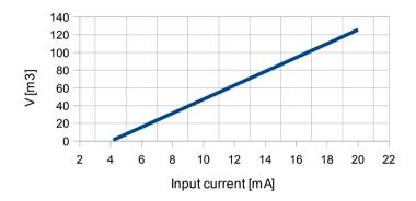
Figure 9.6 The volume characteristic of tank depending on input current in 4÷20mA range.
