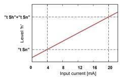
Figure 9.5 The characteristic of level of liquids, gases or solids in tank depending on input current in 4÷20mA range.
