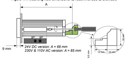
Figure 4.2. Installing of brackets, and dimensions of connectors.
