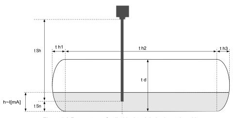
Figure 7.2 Parameters of cylindrical tank in horizontal position.
