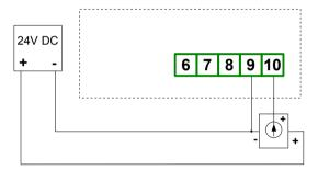
Figure 4.9. Connection of voltage converters
