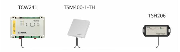
"Star" topology can be used only as a last resort for up to 4 sensors and a total cable length of up to 10 meters.
