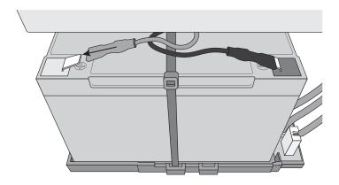
Note: **IMPORTANT:** When putting your Vantage Connect into cold storage, disconnect the red cable
