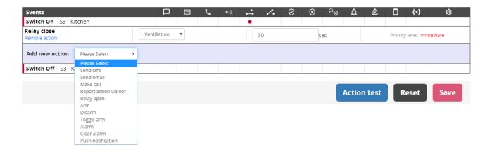
You can assign any number of the following actions to the chosen events in point 4.8. The system is able to manage altogether 100 event-action pairs:
