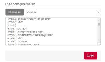
An already existing configuration can be loaded also from file, this time you have to choose the appropriate configuration file from computer, then click on 'Load' button. As an extra function, you can modify the chosen configuration before loading, by clicking on the edit icon.
