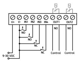
In our example IN1 and IN2 inputs are normally open (NO), while IN3 and IN4 are normally closed (NC) inputs.
