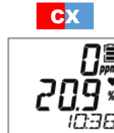
Upper row: CO (carbon monoxide) gas concentration display Middle row: O2 (oxygen) gas concentration display
