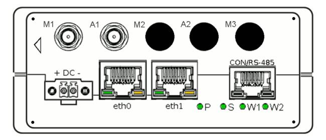
**+ DC-** Power connection. + (VCC) and – (0V/GND) are marked on the
