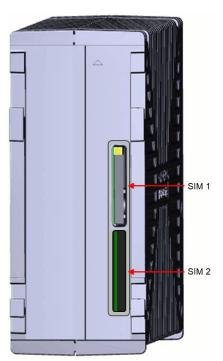
Remove the SIM tray by pressing the yellow button in the "SIM 1" slot with a screw driver.
