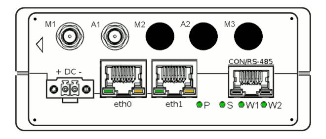
In normal operation mode the LEDs **Power** (P) and **Router Status** (S) are on, as well as the **orange LEDs** of all connected Ethernet ports.
