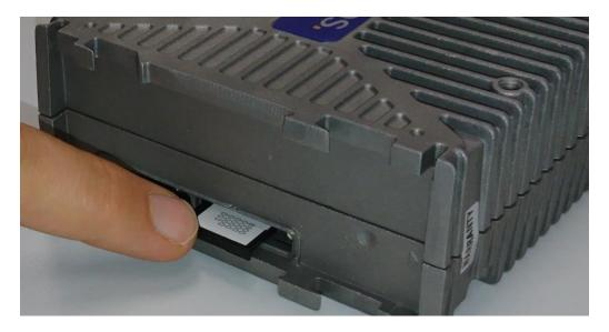
Put back the DIN rail mounting kit after that into the initial position.
