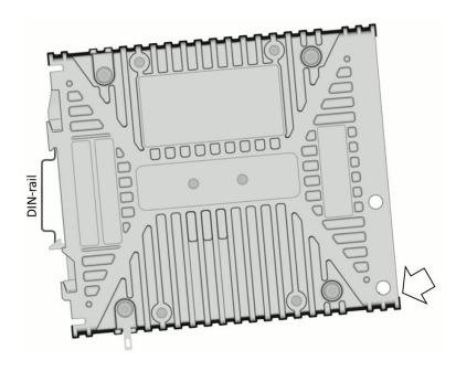
For unmounting push the router up, then remove it from the top of the DIN rail first.
