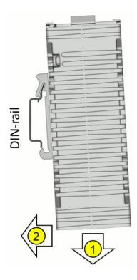
For unmounting push the router down and remove the lower part of the clip from the DIN rail first.
