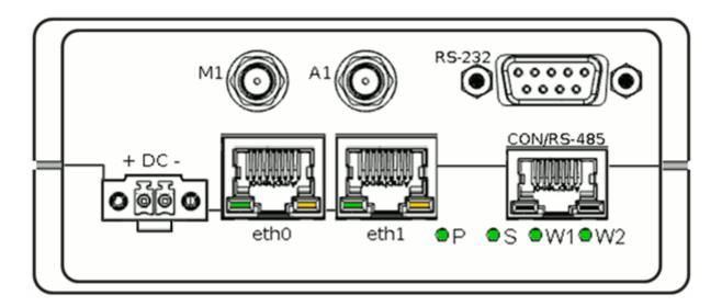
In normal operation mode the LEDs **Power** and **Router Status** are on, as well as the **green LEDs** of all connected Ethernet ports.
