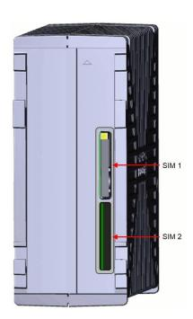
Remove the SIM trays by pressing the yellow button with a screw driver.
