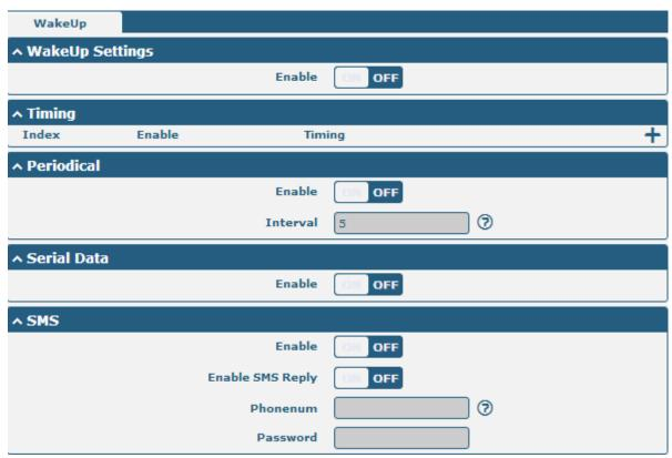
Click on the right side 🕂 of the Timing to add a wake-up time point. Up to 3 can be added.
