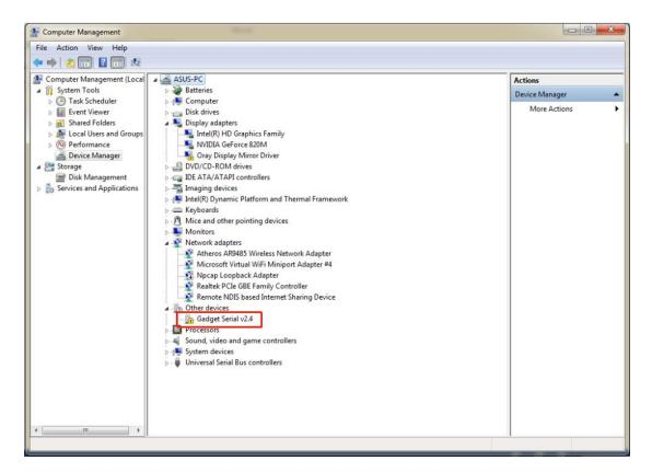
(2) After USB is connected to the PC, check the identified serial port. Different ports of different USB interfaces are different. Right-click and select "Properties" to set the serial port speed to 115200, and click "OK";
