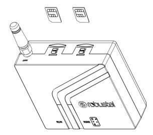
Please confirm before inserting the SIM card. When the SIM card is turned on and the device is configured without the correct PIN, the SIM card is unavailable.
