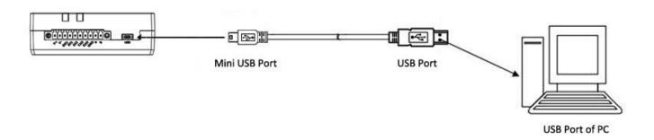
Connect a USB cable to the gateway's mini USB interface to an external controller or computer's USB port
