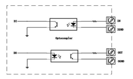
R1520 supports 1 channel DI and 1 channel DO, the internal schematic diagram is as shown above;
