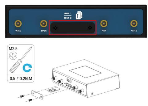
Insert or remove the SIM card as shown in the following steps.
