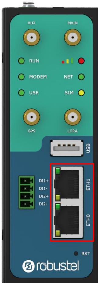
There are two Ethernet ports on R3000 LG, including ETH0 and ETH1. Each Ethernet port has two LED indicators. The yellow one is a link indicator, while the green one is a speed indicator. For details about status, see the table below.
