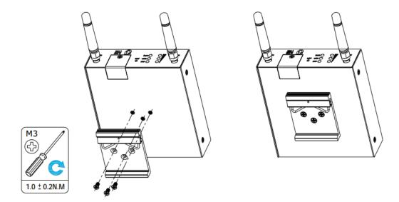
Use 3 pcs of M3\*6 flat head Phillips screws to fix the DIN rail to the router, and then hang the DIN rail on the mounting bracket. It is necessary to choose a standard bracket.
