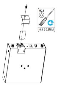
Insert or remove the SIM as shown in the following steps.
