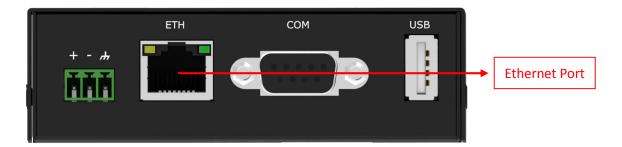
R3000 Lite Router has one Ethernet port with two LED indicators. The yellow one is link indicator and the green one is speed indicator. For details about status, see the table below.
