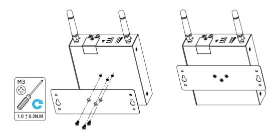
Use 3 pcs of M3\*4 flat head Phillips screws to fix the wall mounting kit to the router, and then use 2 pcs of M3 drywall screws to mount the router associated with the wall mounting kit on the wall.
