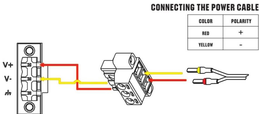
R3000 Router supports reverse polarity protection, but always refers to the figure above to connect the power adapter correctly. There are two cables associated with the power adapter. Following to the color of the head, connect the cable marked red to the positive pole through a terminal block, and connect the yellow one to the negative in the same way. The last step is to plug the power adapter into your socket.
