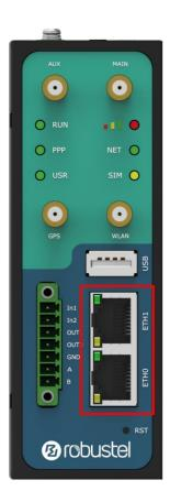
There are two Ethernet ports on R3000 Router, including ETH0 and ETH1. Each Ethernet port has two LED indicators. The yellow one is a link indicator, while the green one is a speed indicator. For details about status, see the table below.
