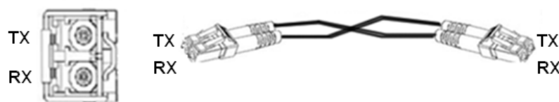
Figure 15 Fiber Connection of an SFP Optical Module
