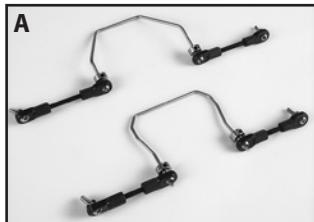
2. Install the links from the front sway bar into the hole closest to the chassis in the front suspension arm (toward the front) (B). Set the sway bar into the groove located on the chassis just behind the shock tower. Thread the included 3x6mm flathead screws into the holes (C) until they touch the bar, and then back off slightly.
