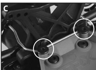
3. Install the links from the rear sway bar into the hole closest to the chassis in the rear suspension arm (toward the front) (D). Set the sway bar into the groove located on the rear bumper mount. Thread the included 3x6mm flat head screws into the holes (E) until they touch the bar, and then back off slightly.
