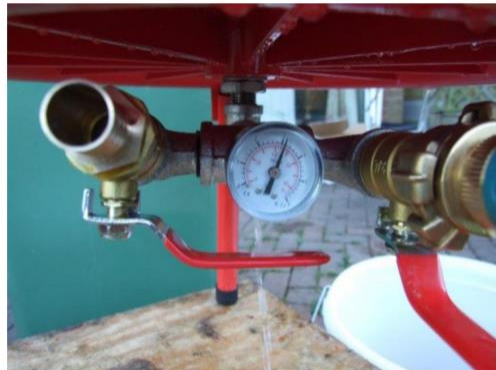
Fig 5. Outlet valve (closed) & pressure gauge
