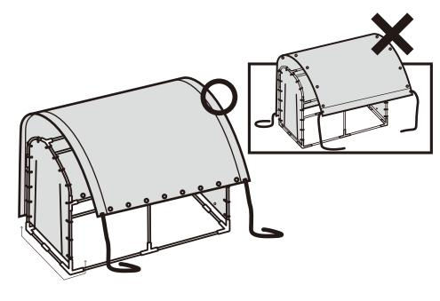
6 Tie one side of the roof cover rope ends on parts #17.
