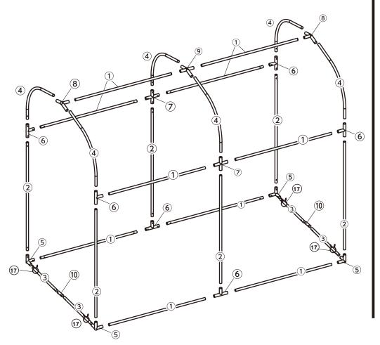
1 Follow below diagram, assembly the basement structure first.
