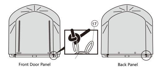
Tie the other side of the roof cover rope end on parts #17 also (drawing A), and then through the door panel eyelet and tight again(drawing B).
