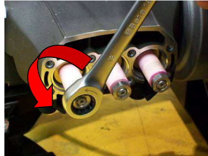
Unscrew the piston lock screw
