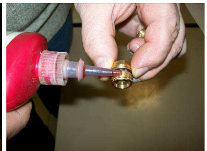
Reassemble the caps using sealing glue type Loctite 542.
