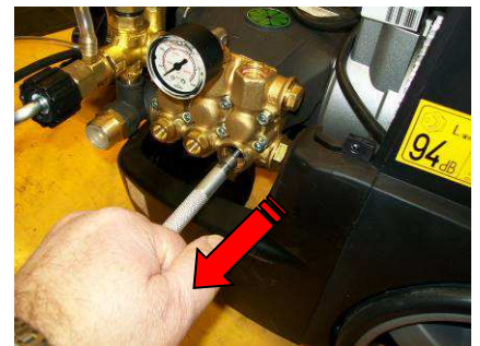
Strip out the valves, use a screw M4 to link and pull out the valve
