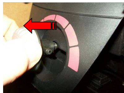
Slide out the detergent tap and replace it if necessary.
