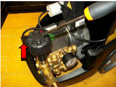
Remove the knob by pulling it out
