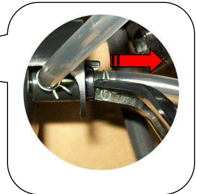
Remove the clips that hold the pipes.
