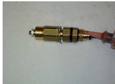
To reassemble the by-pass whole cartridge to the by-pass valve, we recommend the use of Loctite 542.
