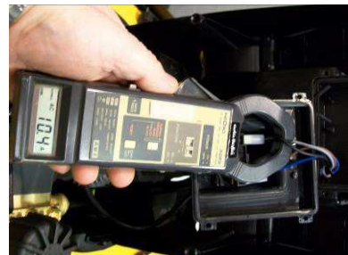
Measured Amperage should be less or equal than Amperage wrote to the machine data plate.
