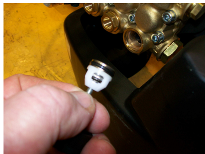
Remove the 6 valve from the pump head and replace them if wear and tear
