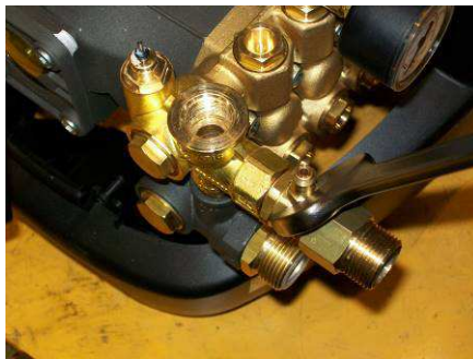
Unscrew the Venturi system.
