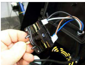
5. Check the main switch contacts continuity using a multimeter, if damaged replace it.
