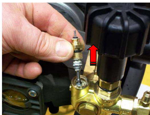
Slide out the piston and its spring, check if parts are wear and tear and if necessary replace them. Lubricate with grease at the reassembly.
