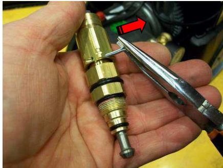
To disassemble the by-pass piston, slide out and remove the locking pin.
