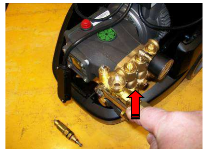
Unscrew the fixation bolt of the by-pass place at the high pressure side.
