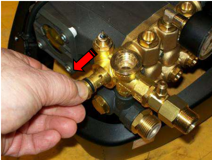
Slide out the fixation bolt of the by-pass
