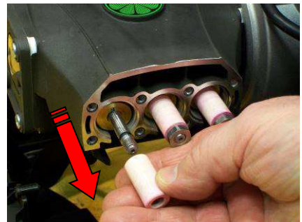
Slide out the damaged piston
