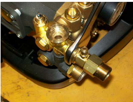
Unlock the nut that avoid the rotation of the outlet fitting.
