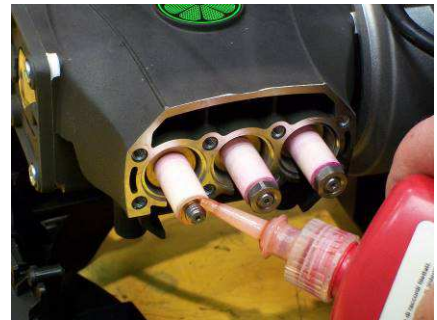
Assemble the new piston and secure the screw with "Loctite 541" glue.
