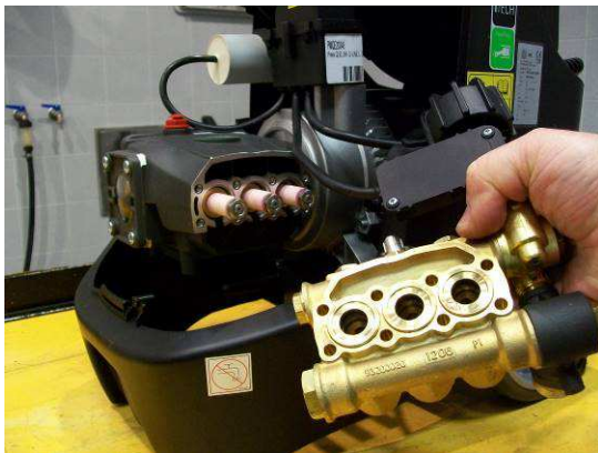
Remove the pump head
