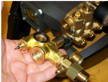
The by-pass valve is so disassembled, if necessary it can be replaced with a new one.
