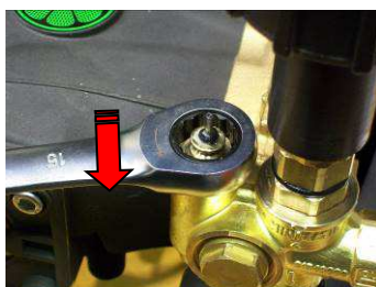
Unscrew the piston that activates the micro-switch
