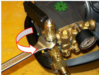
Unscrew the valve cartridge
