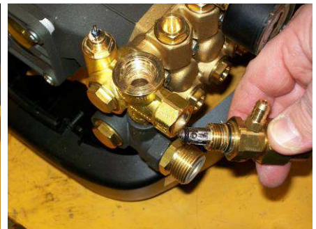
Replace, if necessary, the whole Venturi nozzle and note that the Venturi holds the outlet check valve of the by pass.
