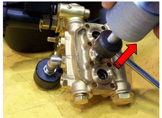
Extract the seals packing using the extractor tool part number PVVR31382.
