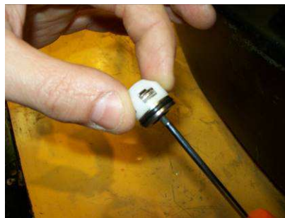
Unstick the valve from its seat pressing gently with a pin.
