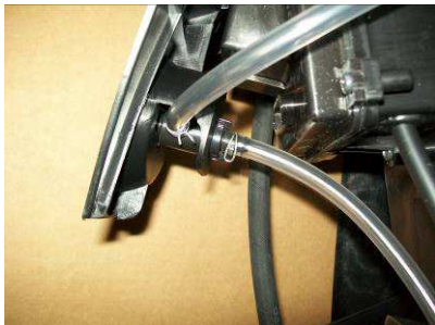
The access to the detergent tap is possible just after the machine cover has been removed.
