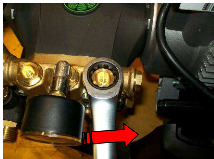
Unscrew the inlet valve caps
