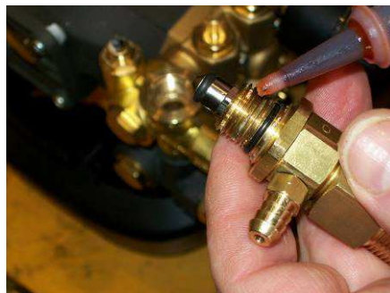
Reassemble the Venturi using a bit of Loctite 542 to seal the threads.
