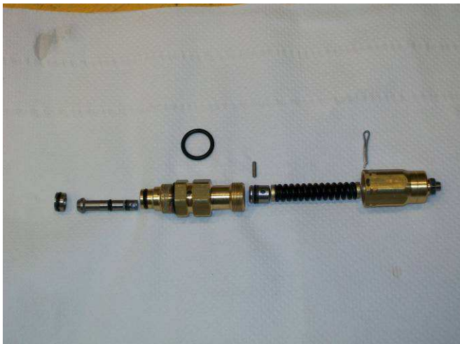
To disassemble the by-pass piston, slide out and remove the locking pin.
