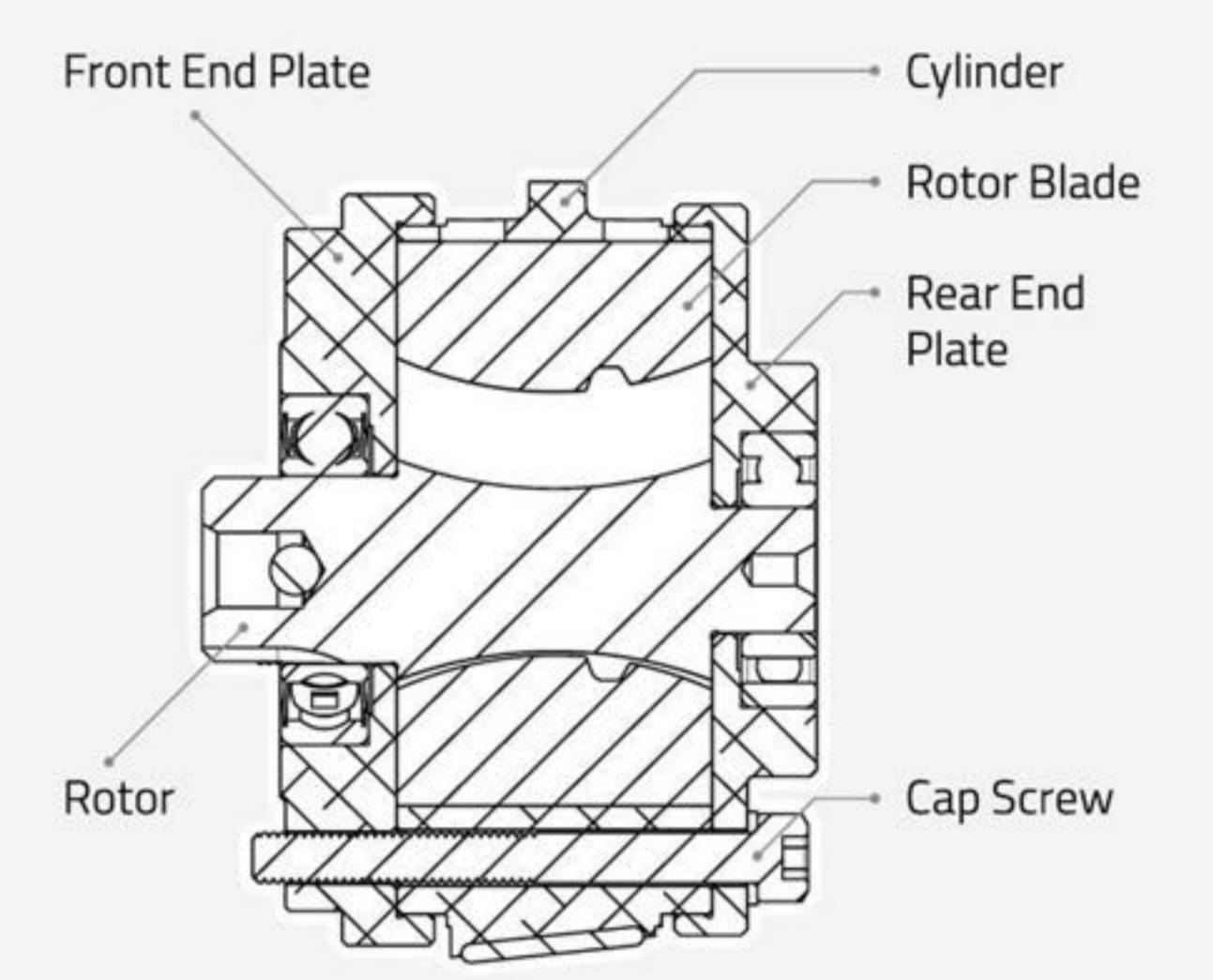
The air motor is a sub assembly is held together with a cap screw, ensuring no misalignment of the end plates — reducing end plate wear, while ensuring no loss of motor power due to air leakage.
