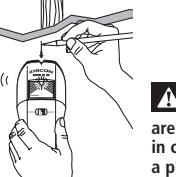
Without releasing the Power Button, continue scanning beyond the marked spot until some Target Indication bars turn off. Slide unit in the reverse direction to locate the other edge of stud.
