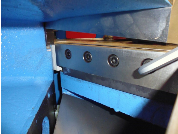
Fig. 21: Unscrewing of the screws of the lower knife
