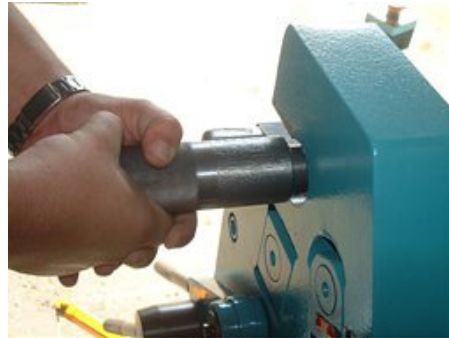
Fig. 14: Release lock of top roller
