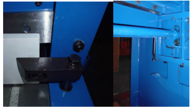
Fig. 9: Workpiece hold-down (left), adjusting screw (right)
