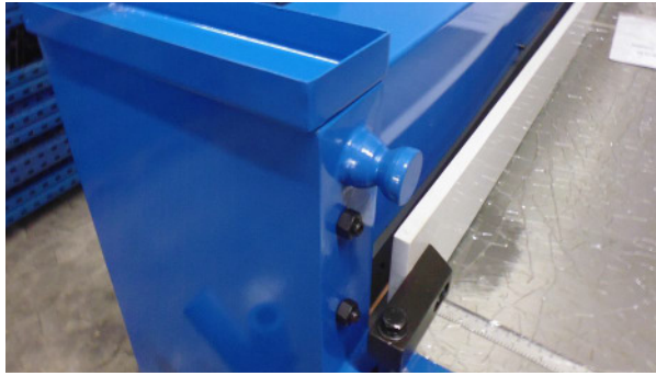
Fig. 6: Adjust cutting gap, nuts for position of the upper knife on the front
