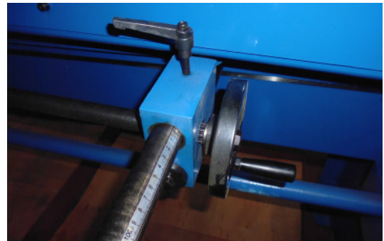
Fig. 10: Adjust rear stop: Clamping screw, handwheel and scale
