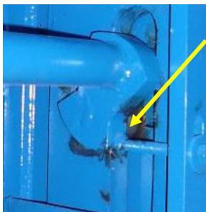
Fig. 8: Lower stop for upper knife
