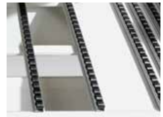
Rollers on arms of pneumatic sheet support
