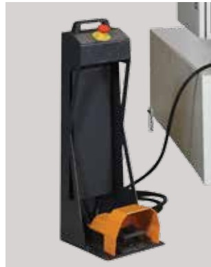
Foot pedal console with emergency stop button and hand grip
