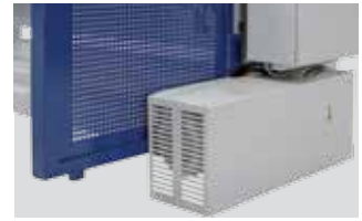
Motor mounted outside the machine frame to leave a totally free area under the table
