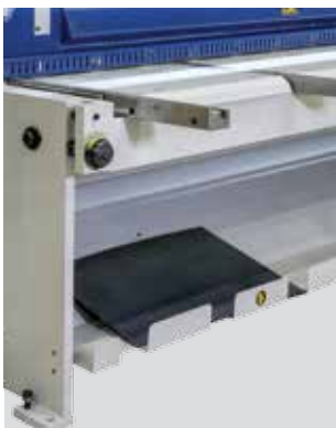
Sheet shute to bring cut plates to the front
