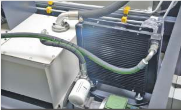
Hydraulic Oil Cooling System
