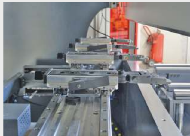
Additional Back Gauge Fingers for 2-3-4-5-6 Axis Back Gauge
