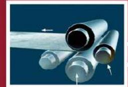
1. Align the plate against the raised rear side roll. Raise the lower roll to pinch the plate. Return the plate to prebending position.
