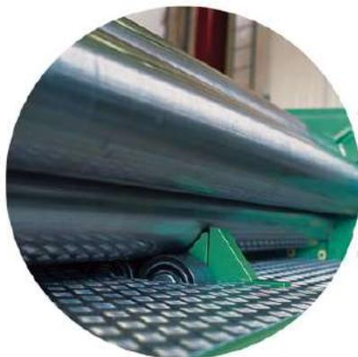
Adjustable support rolls for the lower roll
