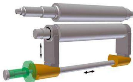
Ensured parallelism on PASS with wedge blocks adjusted by a hydraulic cylinder
